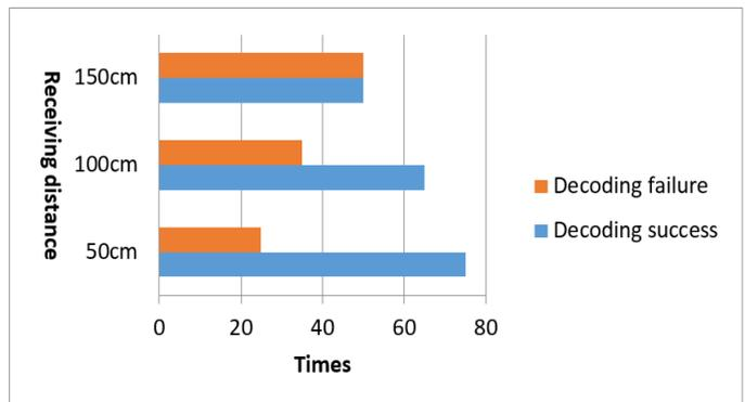
Figure 9. The relation of the receiving distance and decoding result.
