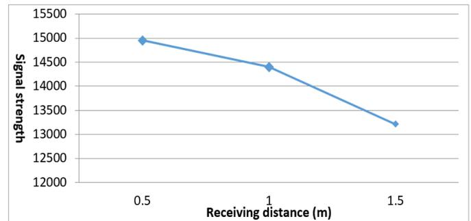
Figure 8. The relation of the receiving signal strength and the receiving distance.
