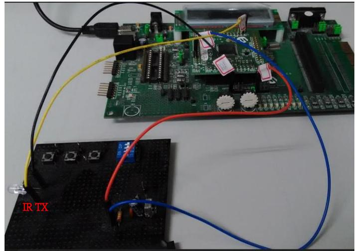
Figure 2. The prototype of IR base station.
