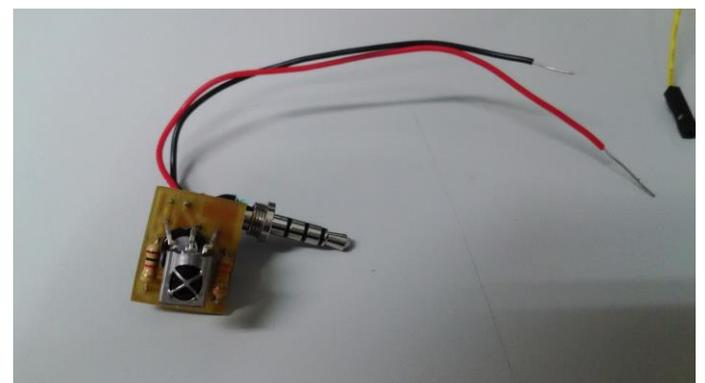
Figure 5. The prototype of IR Receiver dongle.
