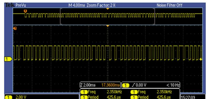
Figure 4. The complete MAC address captured from IR base station.
