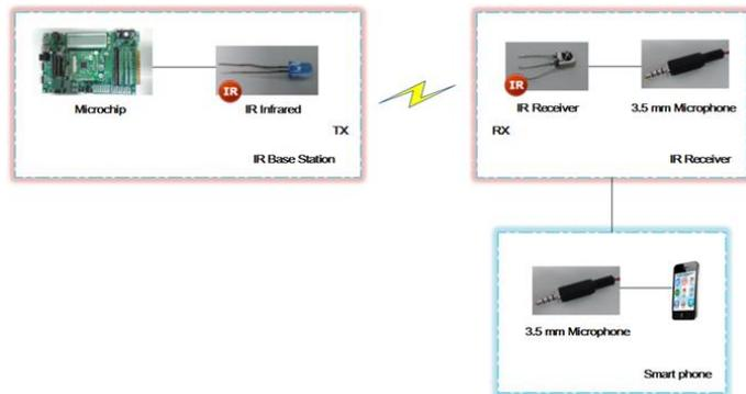
Figure 1. The system architecture.
