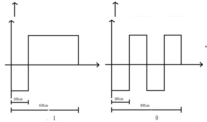
Figure 3. The signals of 1 and 0.
