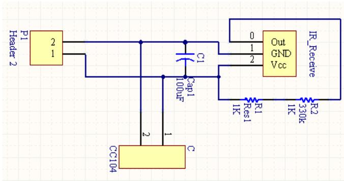
Figure 6. The circuit of IR Receiver dongle.
