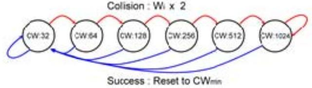
Figure 1. DCF algorithms of Markov Chain Model.
