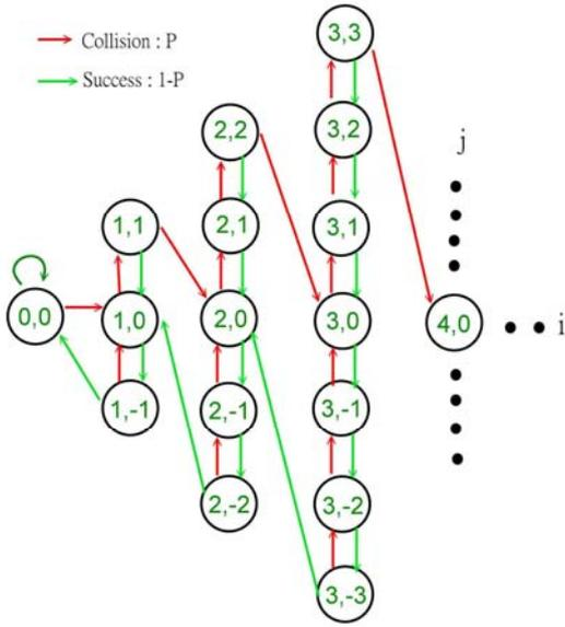
Figure 4. OAB algorithms of Markov Chain Model.
