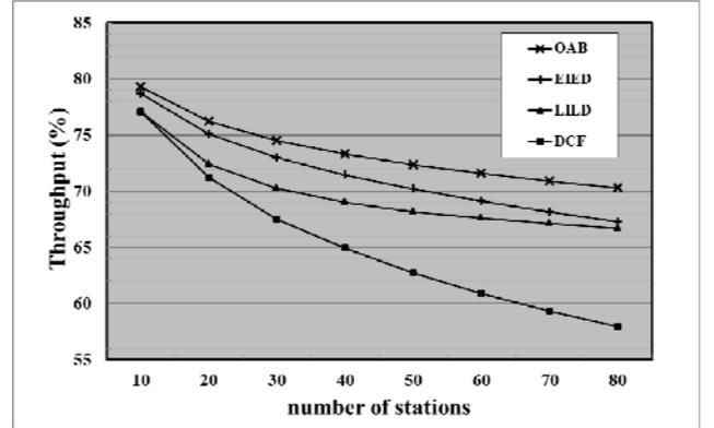
Figure 5. Throughput of different backoff schemes.
