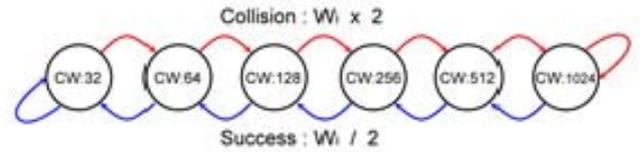
Figure 2. EIED algorithms of Markov Chain Model.
