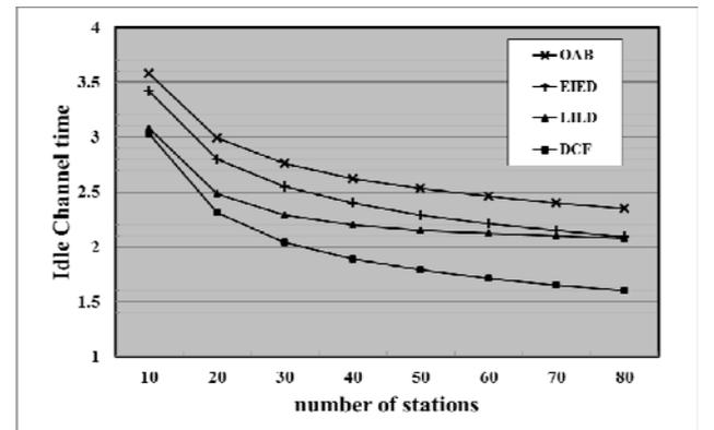
Figure 7. Idle channel time of different backoff schemes.
