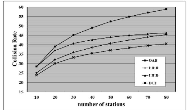
Figure 6. Collision rate of different backoff schemes.
