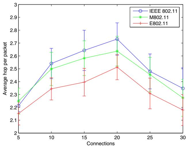
**Fig. 4** The average number of hops for a packet that successfully reached the destination node for various number of connections
