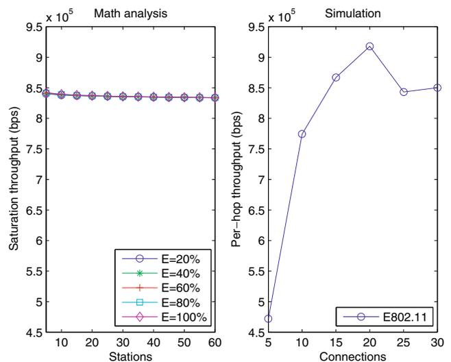
**Fig. 11** Comparison of analytical model and simulation for E802.11
