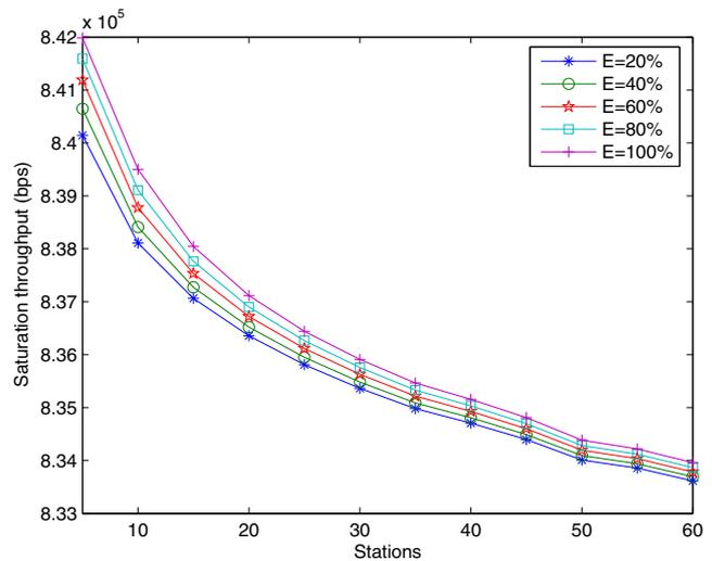
Fig. 2 Saturation throughput for energy-efficient 802.11 analytical model
