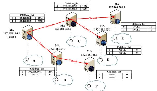
Fig.3 Overlay tree setup by type-1 MA
