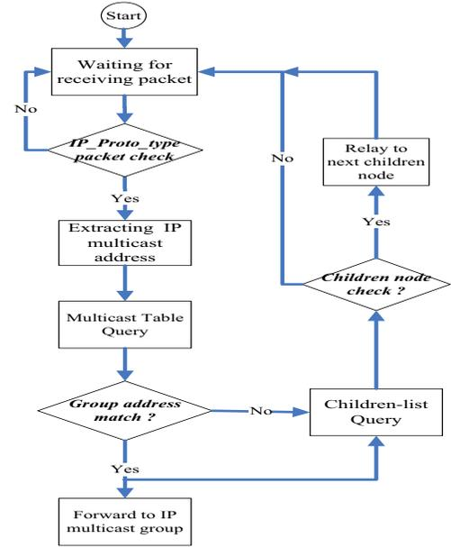
Fig.5 Two-tier multicast routing and forwarding control procedure
