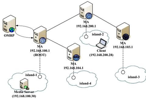
Fig.6 Integrated MA network test environment
