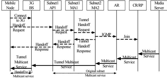
(c) MN vertical handoff multicast service from WLAN AP1 to 3G BS via tunnel between MA1 and MA2
