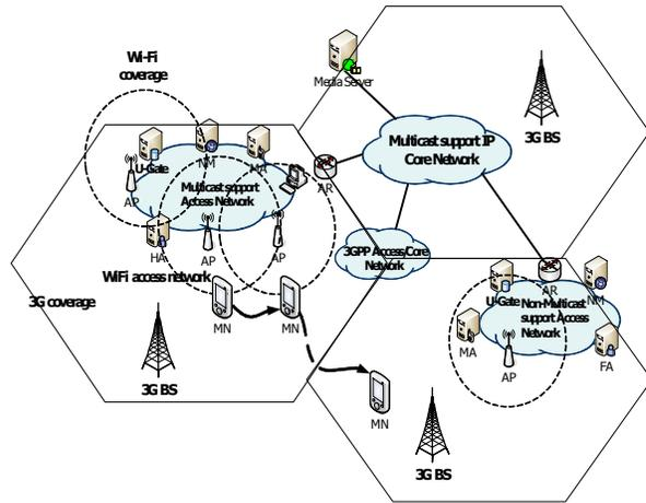
Fig. 1. Hybrid wired/wireless network environment
