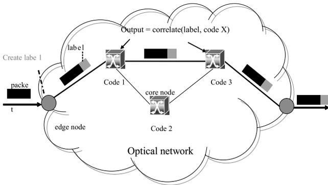
Fig. 2 An optical CDM label switching system.
