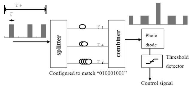
Fig. 4 Simplified optical correlator architecture.
