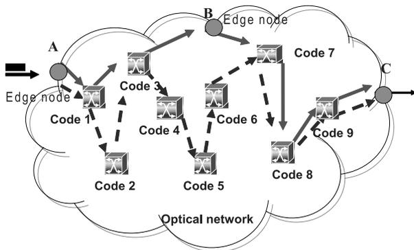
Fig. 6 Route AC is divided into two routes, AB and BC.
