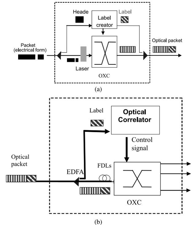
Fig. 3 (a) Ingress edge node architecture. (b) Optical switch (core) node architecture.
