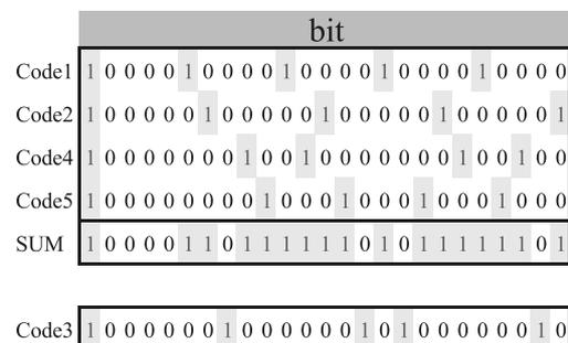
Fig. 7 Example of prime code, label is made up of 1, 2, 4, 5.
